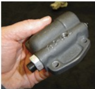
The spring loaded relief valve opens when the oil pressure reaches its limit.
