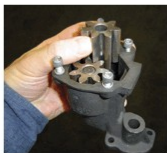
High-Volume oil pump gears will push more oil (20-25%) at the same rpm as a stock pump.
