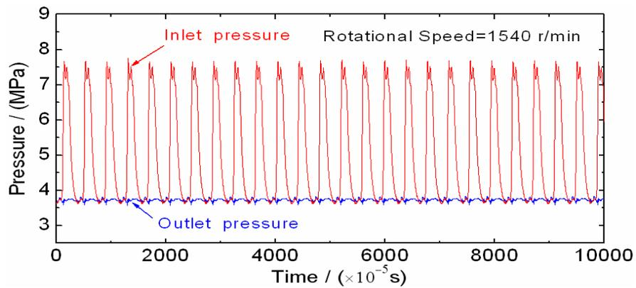
Fig.5 P-T diagram in working condition of II
