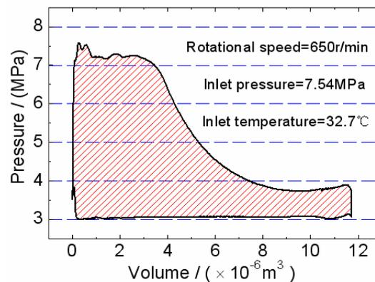
Fig.9 P-V diagram in working condition of III
