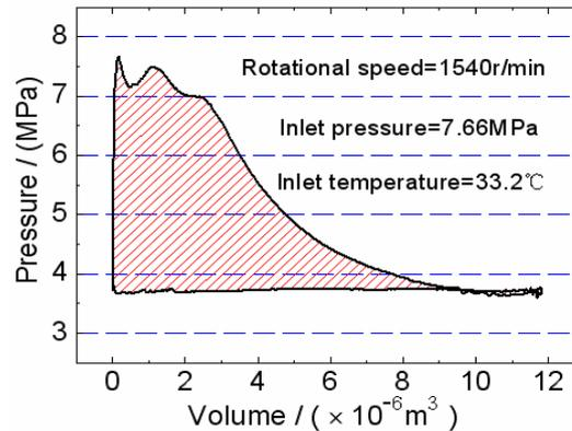
Fig.8 P-V diagram in working condition of II
