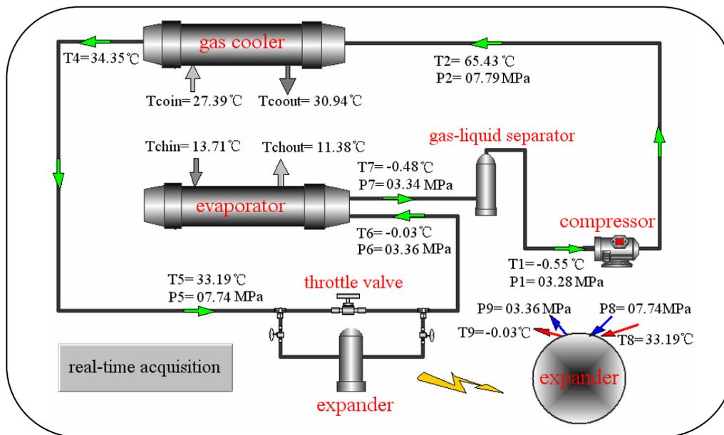
Fig.3 Schematic view of P-V diagram of rolling piston expander test rig system
