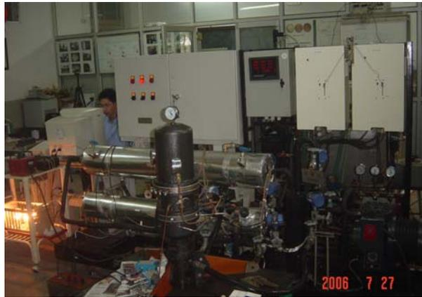
Fig.1 Water-water heat pump system with expander
