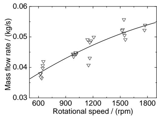
Fig.11 Influence of rotational speed on mass flow rate of expander
