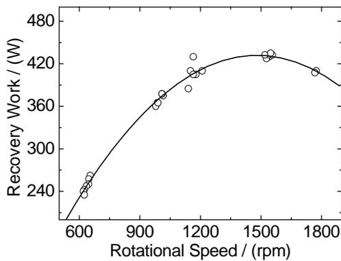
Fig.12 Influence of rotational speed on recovery work of expander in practical working conditions
