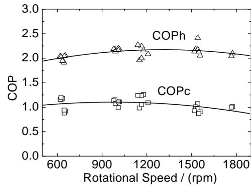
Fig.13 Influence of rotational speed of expander on COP of system
