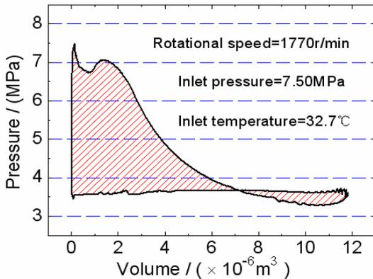
Fig.7 P-V diagram in working condition of I
