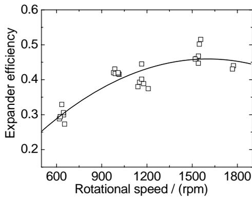
Fig.10 Influence of rotational speed on efficiency of expander
